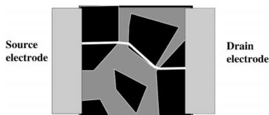
Fig. 5 Schematic model of the conductivity hierarchy in polycrystalline samples. Highly ordered domains are shown in black, being separated by disordered areas shown in gray. Charge carriers will follow a path minimizing the path length in the disordered areas as indicated by the white line.
